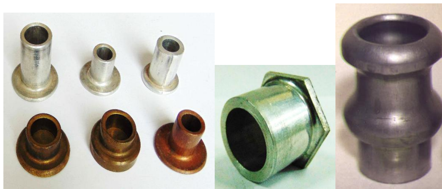
Fig. 12. Hollow parts produced by radial-backward extrusion
